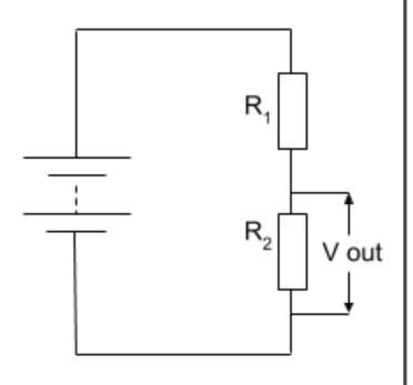
**Variable resistors** in a potential divider are used to change the voltage supplied to something to a suitable voltage without using a transformer. However, this method wastes power.
